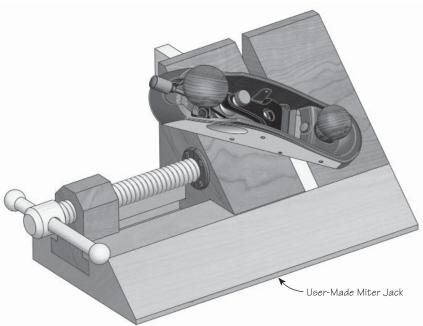
Figure 6: Shooting with a user-made miter jack.
