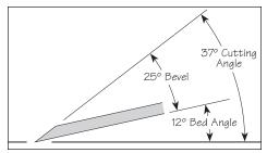
Figure 4: 25° blade geometry.
