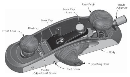
Figure 1: Veritas Miter Plane components.
